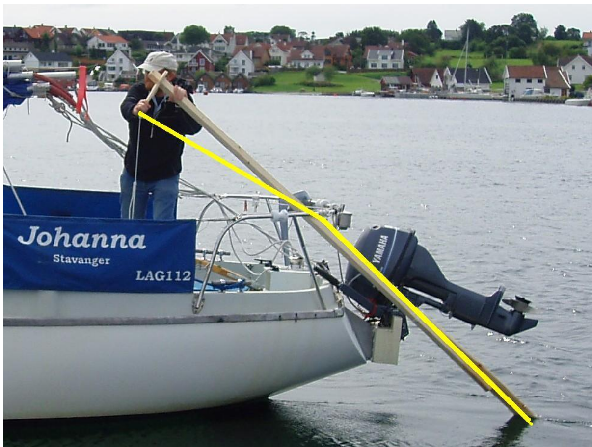
2.8.2008 This re-touched photo illustrates how the wrench, with the lanyard fitted to its tip, leads to natural twisting of the yuloh's handle. ("virtual bend").
