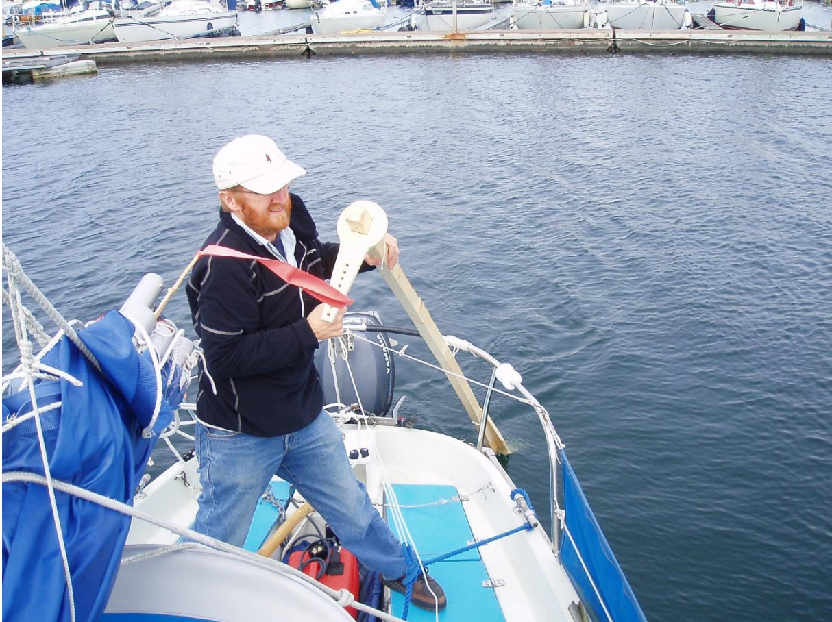
4.8.2008. The lanyard was trial-fastened in several positions on the wrench handle - note the number of holes drilled for it.
